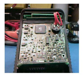
Step 3. Clean socket holes from excess solder. Use either de-soldering braid or de-soldering suction tool.
