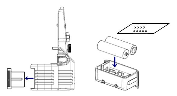
To replace the batteries, separate the battery tray from the pump: unscrew the screws on the front and pull the battery tray out of the unit.
