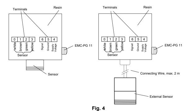
The supply voltage for the transmitter (terminal 4) is 10...32 V DC.
