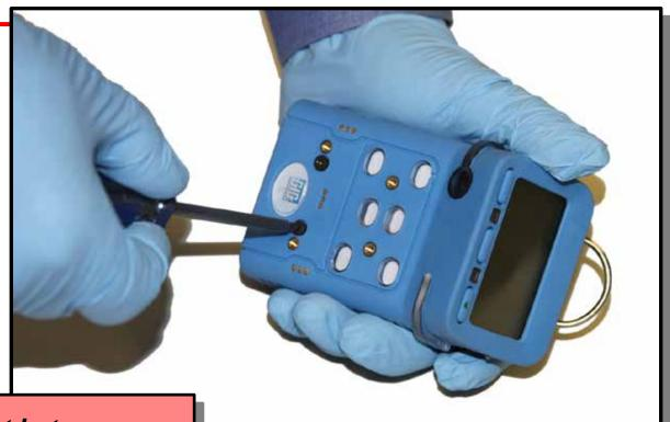
Note: Direct contact between fingers and PID lamp, electrodes and other components can leave oils and contaminants behind that can degrade performance
