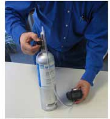
Figure 1: Performing a functional "bump test" by exposing the instrument to test gas takes only a few moments to perform.
