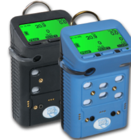
Figure 1: Multi-sensor portable instruments almost always include a sensor for measurement of combustible gas. The G460 is capable of being equipped with sensors designed to measure up to six different atmospheric hazards at the same time.
