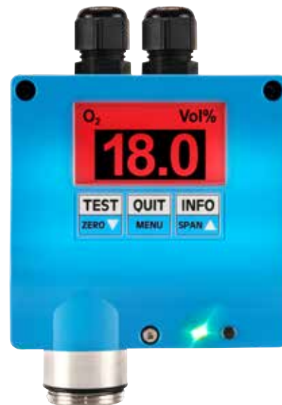
ZD22 D transmitter with display, touch keys and acoustic alarm
