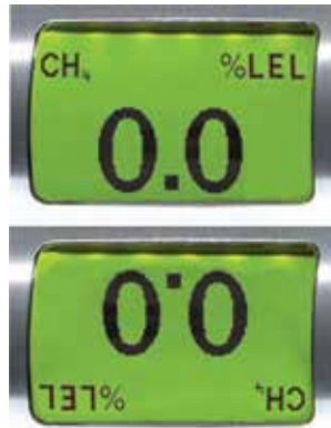
Figure 5: The high contrast easy-to-read display can be flipped 180° for visibility in any position.
