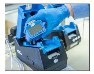
Make sure that the gas detector has been properly sanitized before taking it to a common area, or handing it off to another worker.
