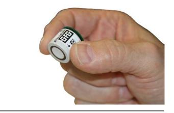
Larger sized sensors have more room for internal filters. The larger size of the sensing electrode and greater volume of electrolyte make them harder to destabilize as well.
