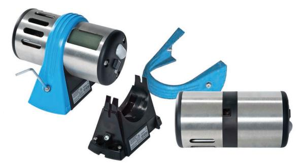
The sensor head assembly of the low power "Ex i" certified IR-29 transmitter can be removed and replaced even when the transmitter is located in Zone 0, gas group IIC, temperature class T4 hazardous locations. Being able to remove and replace the head without needing to declassify the hazardous location makes it easier to perform maintainenance procedures such as calibration and repair.
