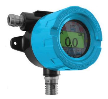
The CC-33 is a fixed system gas transmitter equipped with a catalytic LEL sensor. The transmitter is certified as a flameproof "Ex d" device for use in Zone 1, gas group IIC hazardous locations.
