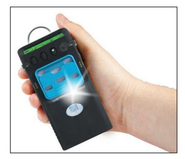
The G999 is a compact, one to six gas atmospheric monitor with optional wireless communication used to transmit realtime monitoring results to a remote collection point. The instrument is certified as an intrinsically safe "Ex i" device for use in Zone 1, gas group IIC, temperature class T4 hazardous locations.
