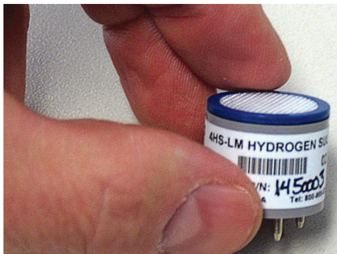
Figure 1. An electrochemical H 2 S sensor module.
