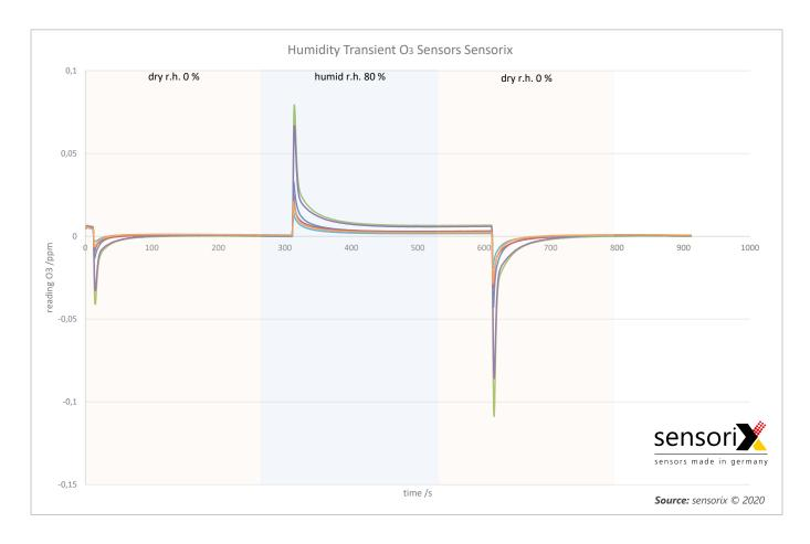
The chart shows the effects of a sudden change in humidity on the reading. You can see how quickly the sensor recovers, and how the positive and negative components in the response balance out to zero with regards to the exposure calculations. This is typical for ozone sensors. However, please note that O3 sensors from other
