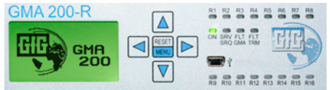
User interface of the GMA200-RTD with display, push buttons, status LEDs and USB port.
